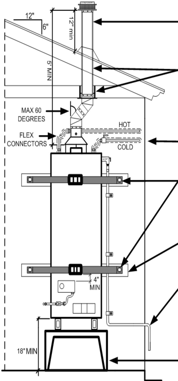
Venting for the water heater shall be Type B (double wall) vent pipe and shall terminate at least 5 feet above the draft hood or flue collar and at least 12" above roof. (steeper pitched roofs will require additional clearances)
